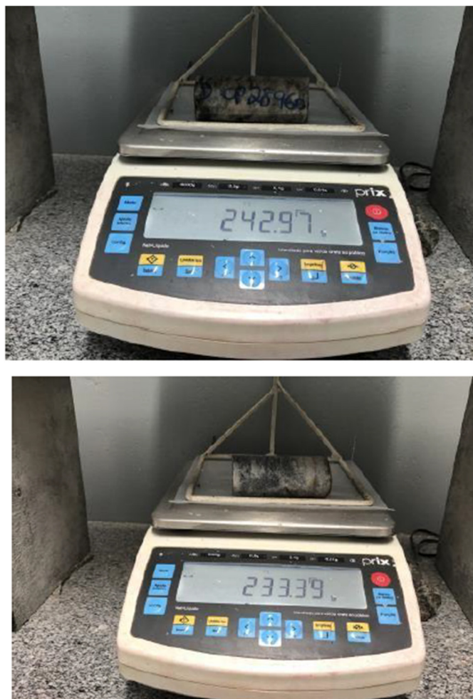
Figure 10-5: Density testing procedure (Ero Brasil, 2022)
