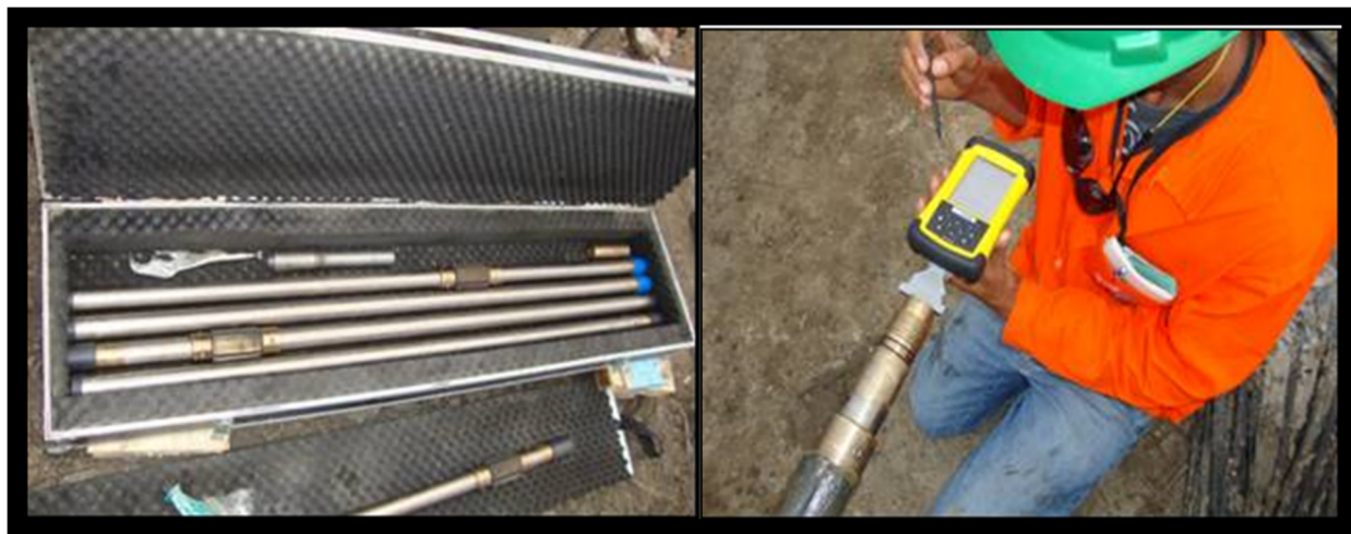
Figure 10-3: Maxibor equipment preparing for drill hole deviation readings (Ero Brasil, 2022)
