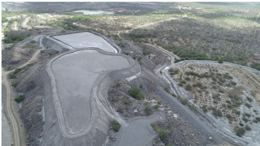
Figure 20-6: Photograph of Co-disposal Method on completion of Deposition (Ero Brasil, 2019)
