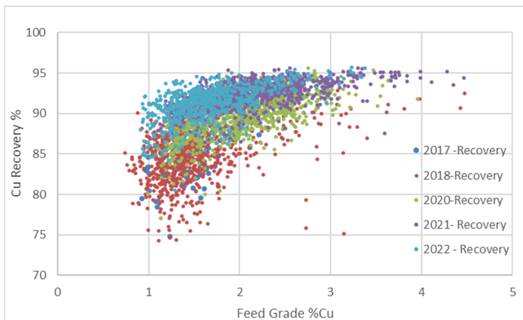
Figure 13-4: Grade Recovery comparison from 2017 to 2022 (Ero Brasil, 2022)
